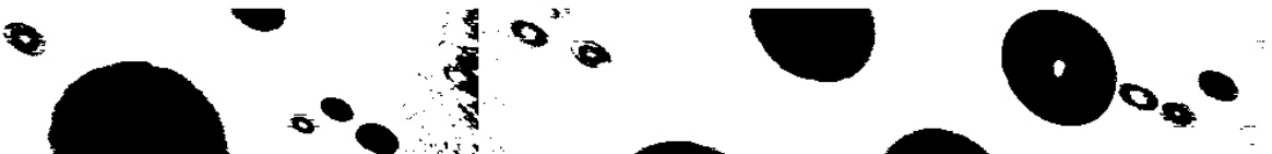
Figure 1: Typical images of natural precipitation drops and spurious images from splashing of drops on the probe. The white space representing distances between images has been eliminated.
