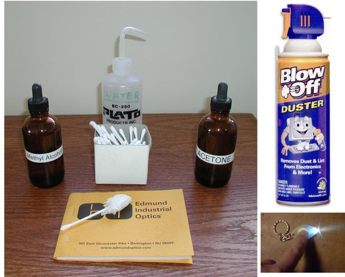
**Figure 4.1.** Items required for window cleaning
