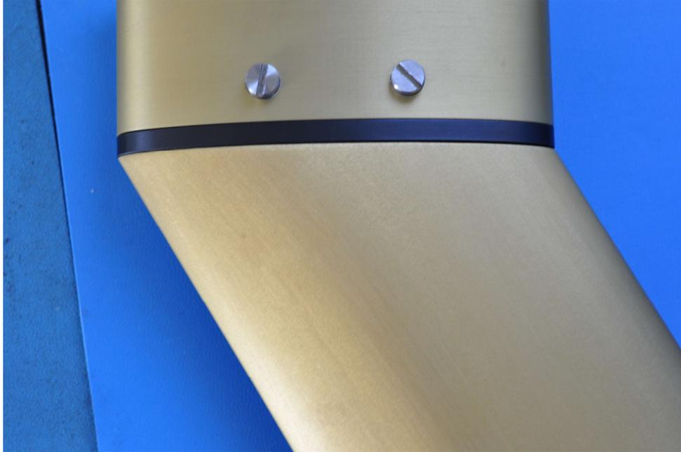
**Figure 5.10:** Mounted FCDP with Custom Bolts
