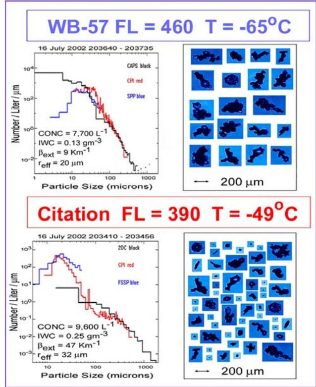
Figure 7. PSDs, CPI images, values of total particle concentration (conc), ice water content (IWC), extinction coefficient ( $\beta_{\text{ext}}$ ) and effective radius ( $r_{\text{eff}}$ ) derived from the composite PSDs for two levels in an anvil studied in Florida during the CRYSTAL-FACE experiment.
