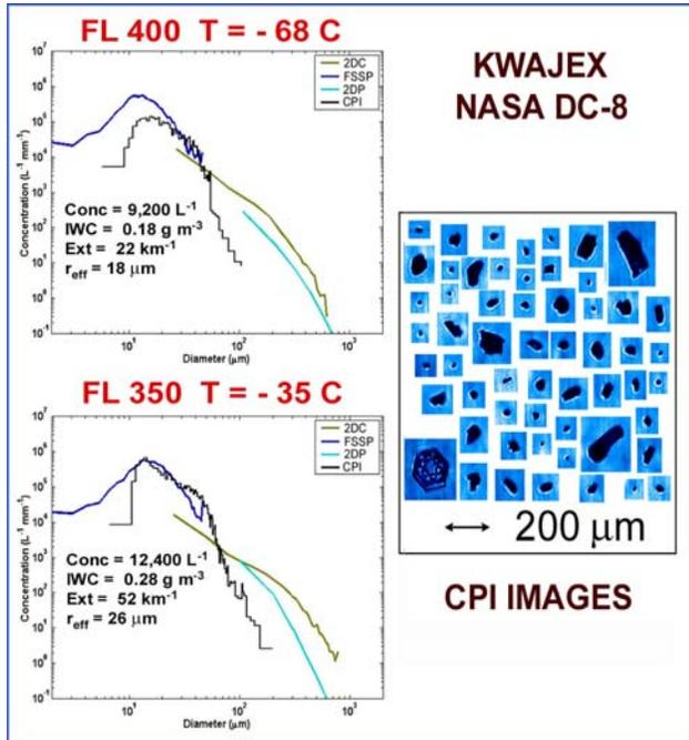
Figure 8. PSDs, CPI images, values of total particle concentration (conc), ice water content (IWC), extinction coefficient ( $\beta_{ext}$ ) and effective radius ( $r_{eff}$ ) derived from the composite PSDs for two levels in an anvil studied near Kwajalein during the NASA TRMM KWAJEX experiment.
