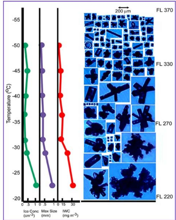
Figure 2. Vertical profile showing examples of CPI images and microphysical data in a deep cirrus cloud (11/16/98). The values of ice particle concentration (Ice Conc), maximum particle size (Max Size) and ice water content (IWC) are 10-s (15 km) average values.
