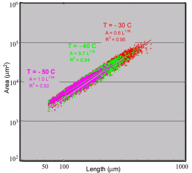
Figure 3. Plot of CPI particle length versus particle area. The data points are color-coded as a function of temperature for the 13 cirrus clouds shown in Table 1. Best fit equations and correlation coefficients are shown for each temperature.
