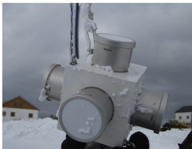
Fig. 2. NILU-CUBE moderate bandwidth filter instrument consisting of six sensors mounted on the faces of a cube.
