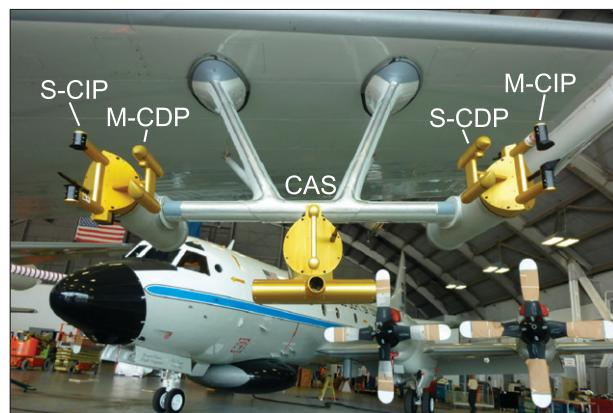
FIG. 1. Cloud probe instruments used during CalNex, labeled by acronyms as defined in Table 1. Wingtip location is toward the right. Another NOAA WP-3D aircraft is visible in the background of the image.
