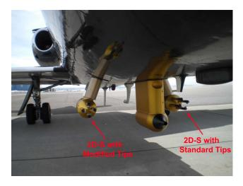
**Fig. 3.** Photograph showing the SPEC Learjet used in the SPARTICUS project with two 2D-S probes, one with tips modified to reduce shattering, and the other with standard tips.
