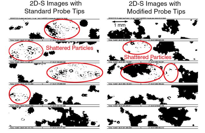
Fig. 5. Examples of 2D-S images from two 2D-S probes flown side-by-side on the SPEC Learjet (Fig. 3) during the SPARTICUS project, one probe had standard 2D-S probe tips (left) and (right) the other with tips modified to reduce the effects of shattering.
