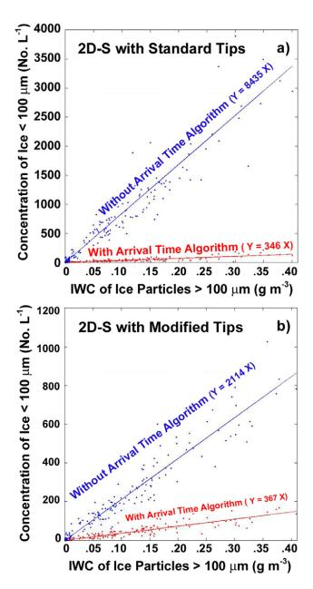
Fig. 7. Scatter plots of the concentration versus ice water content of ice particles  ${<}100\,\mu m$ . Data collected in large ice aggregates with two 2D-S probes installed side-by-side on the SPEC Learjet (Figs. 3–6). One probe (a) had standard probe tips and the other probe (b) was equipped with probe tips modified to reduce shattering. Effect of the arrival time algorithm to remove shattering is shown on each plot.
