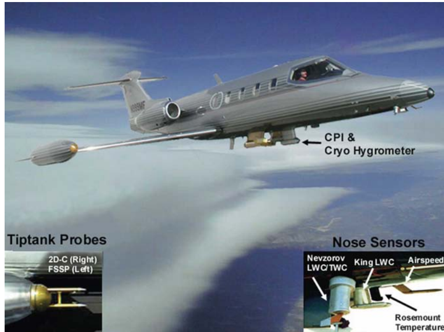
FIG. 1. Photograph of the Learjet showing placement of sensors used in this research. See Table 1 for details on the sensors.
