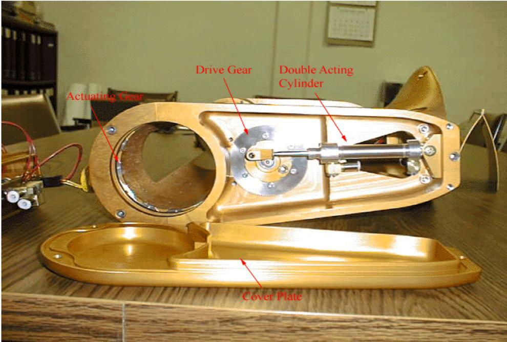
**Figure 24.** Details of drive mechanism for cloak tube.
