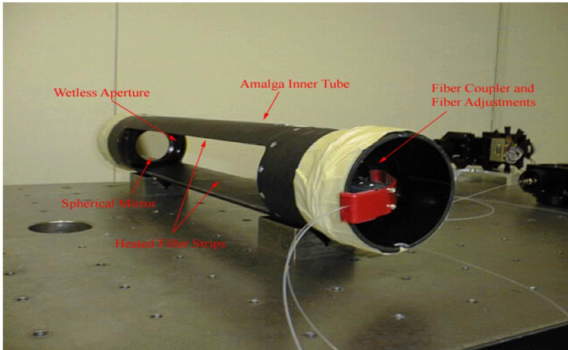
**Figure 17.** Extinctionmeter Herriott Cell / Optical Bench
