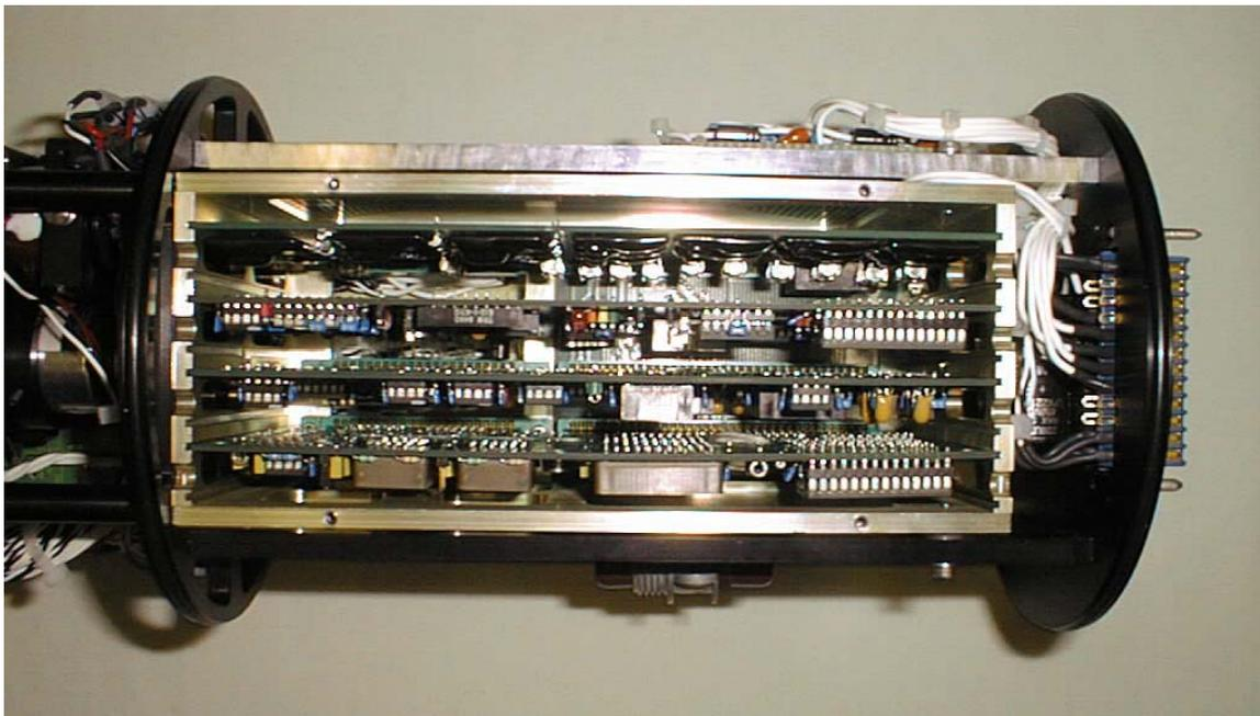
**Figure 29a.** Electronics card set in card cage.
