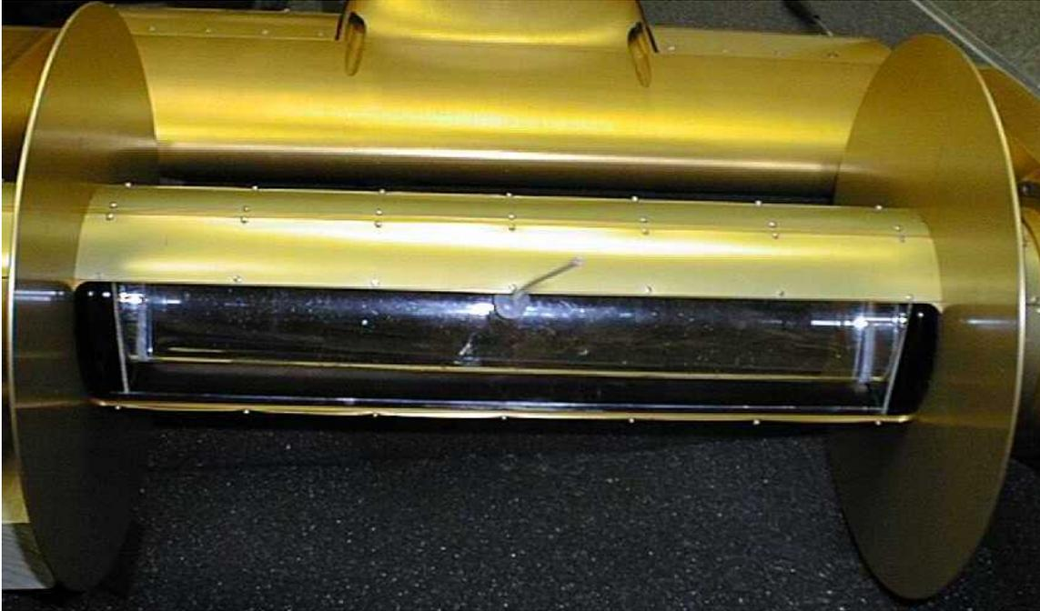
**Figure 82.** Measurements of water turbidity were made by inserting a water-filled, clear acrylic cell into the extincniometer optical path.
