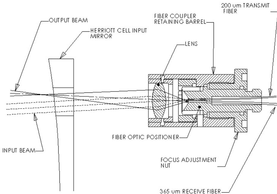
**Figure 13.** Herriott cell to fiber coupling assembly.
