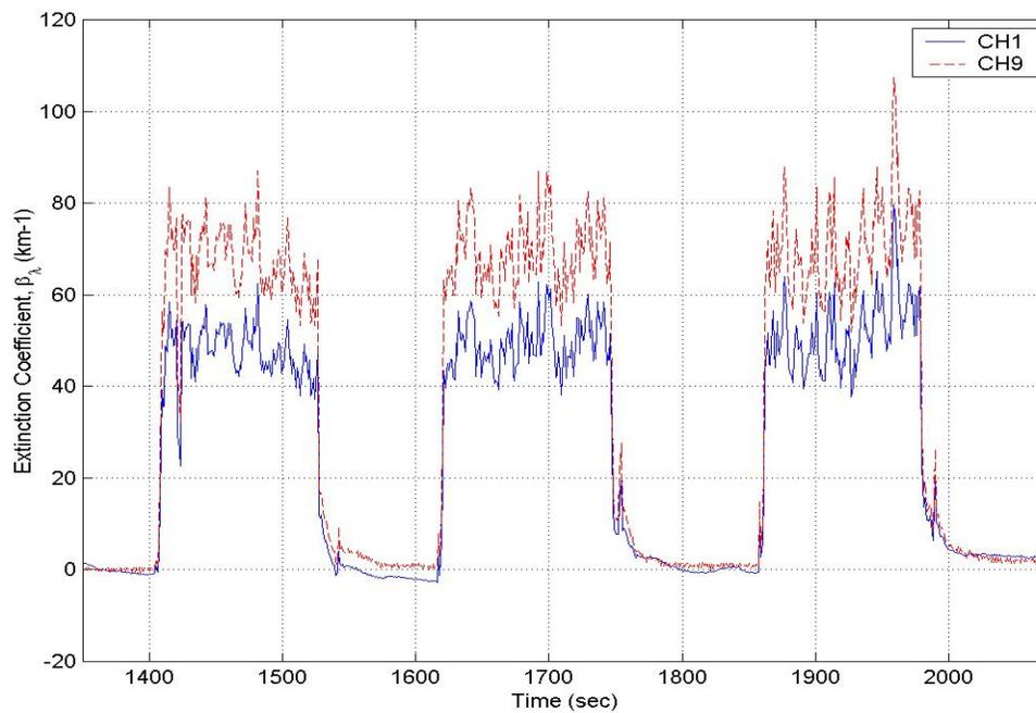
**Figure 39.** Repeatability of Extinguimeter in PMS wind tunnel. Note that the signal returns to the baseline after spray is turned off, indicating that the mirrors are free from contamination.
