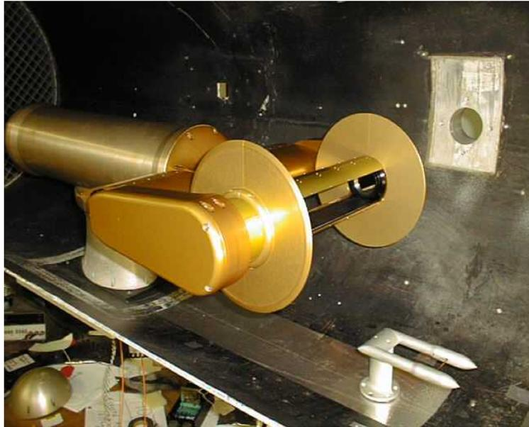
**Figure 38.** Extinguimeter sample head in wet wind tunnel during second round of tests with turbulence fences installed.
