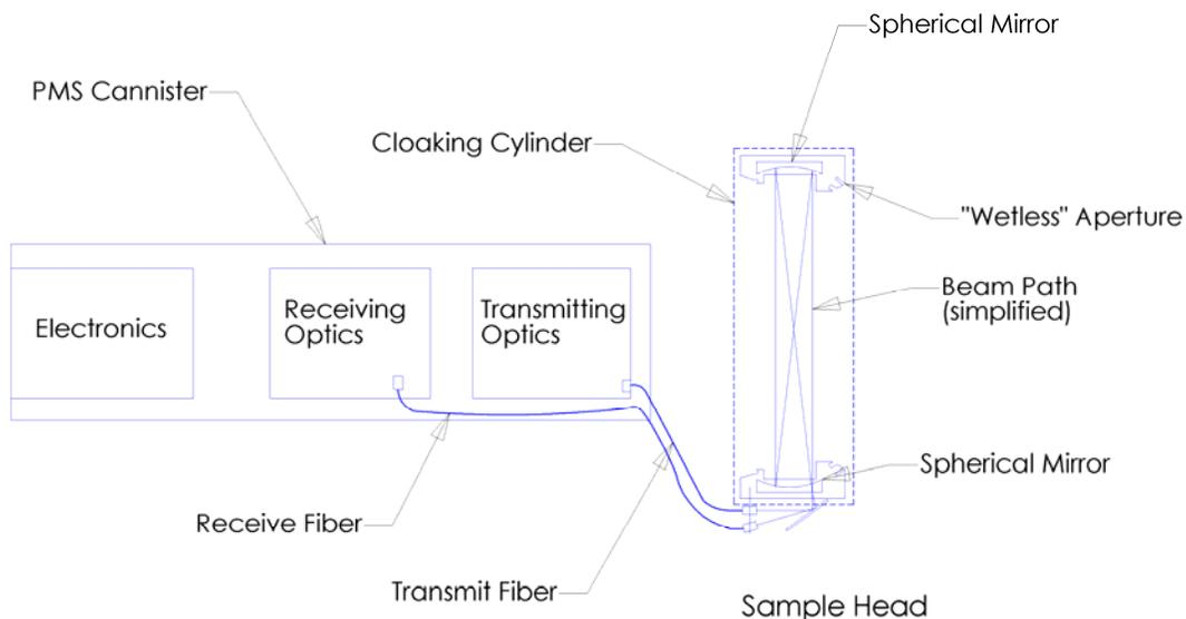
**Figure 10.** Functional layout of extincniometer subsystems.
