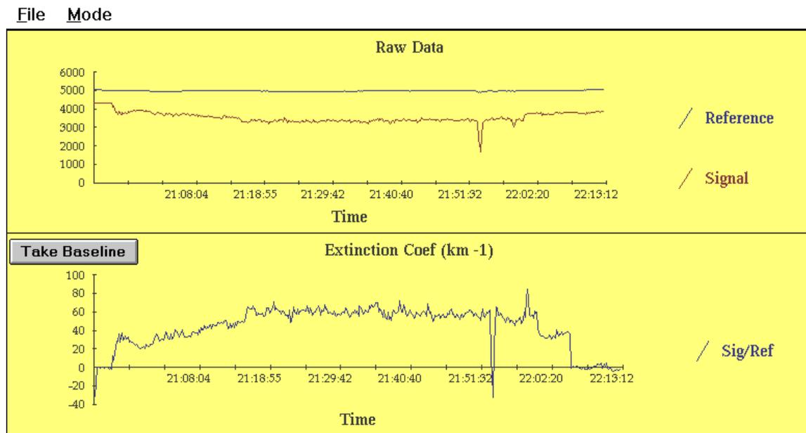
**Figure 3.** A screen print from the real-time display of parameters from the cloud extinction meter. The portions where extinction coefficient is near zero at the beginning and end of the time series are the result of “cloaking” to measure baseline. The negative spike is when a technician put his hand in the sample volume.
