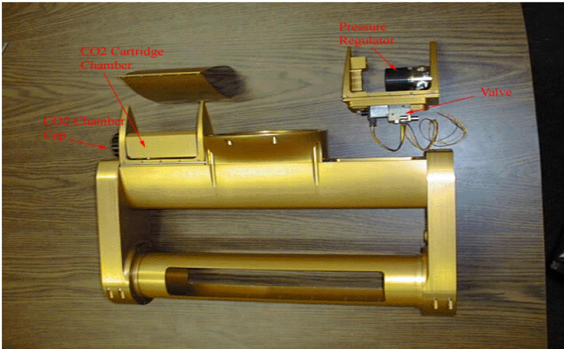
**Figure 25.** Location of cloaking system pneumatic components.
