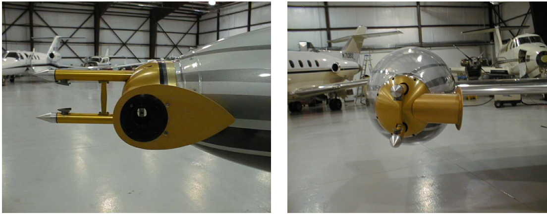
Figure 41. Side and head on views of transmissometer retroreflector shroud.
