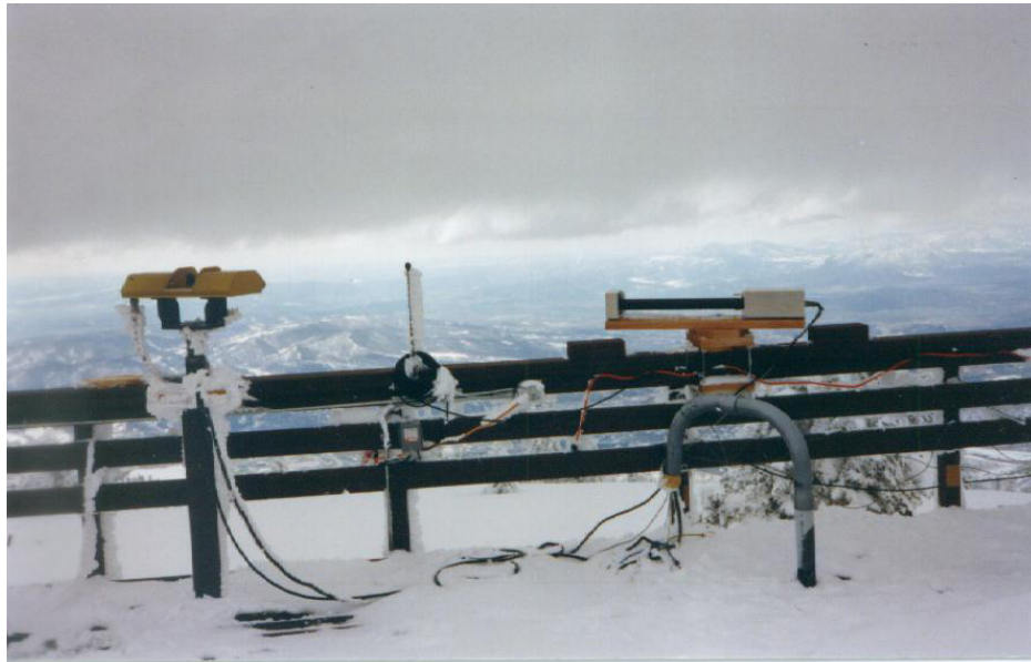
Figure 2. The SPEC automatic cloud spectrometer (ACS)(left) and the cloud extinction meter (right) mounted on a rail on the roof of Storm Peak Observatory.
