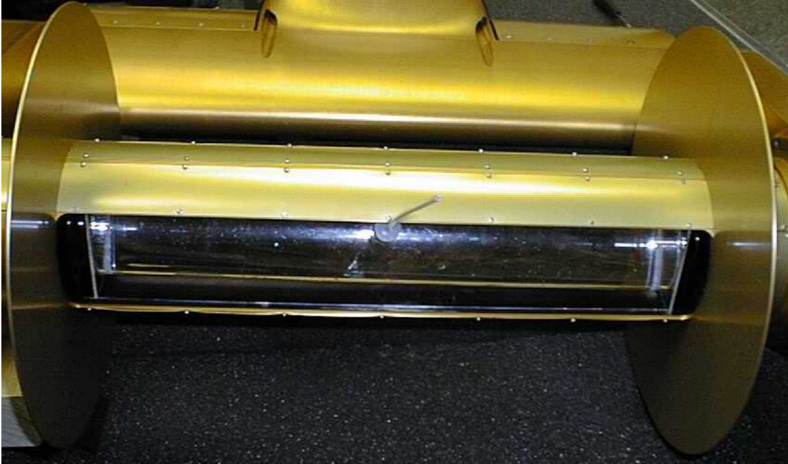
Figure 82. Measurements of water turbidity were made by inserting a water-filled, clear acrylic cell into the extincitometer optical path.
