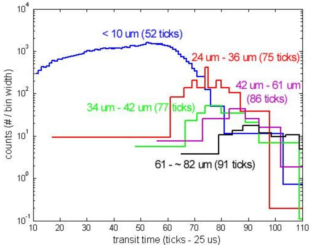
Figure 8: Data from 22 December 2009, 17:08:20-17:10:20 (FSSP time). Transit time distributions for various size ranges created after the DOF rejection step, without shattering removal. The size ranges and location of the peaks are indicated.
