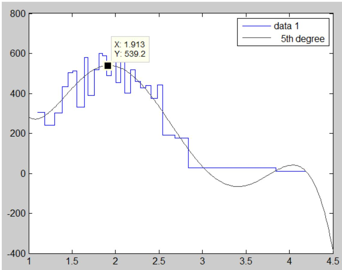
Figure 10: 120904162508 signal distribution after the half peak transit time versus full transit time qualification step (i.e. just before the final transit time qualification steps) and after the small end was removed by using the noise filter. A fifth degree poly fit is also shown that was used together with the data tip tool to identify the value at the peak.
