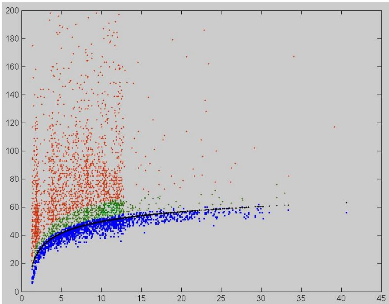
Figure 5: Half peak transit times versus size for the ICE-T FCDP 110712175445\_frm\_5228\_to\_5236\_PBP data after slit comparator qualification in red. Black data shows the ideal transit times estimated from sizes while green and blue overlays show those events also size dependent transit time qualified by the older and new criteria respectively.
