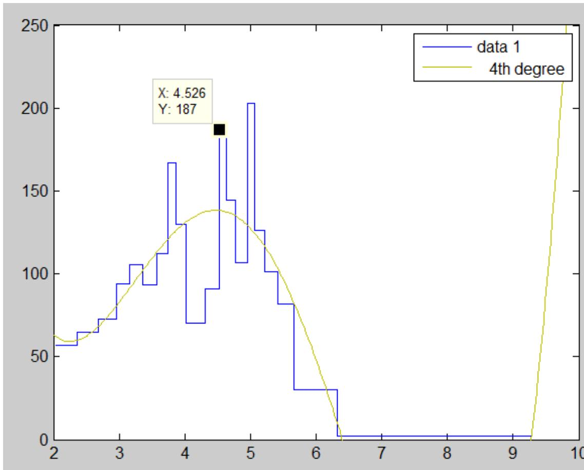
Figure 14: 120904162807 signal distribution after the half peak transit time versus full transit time qualification step (i.e. just before the final transit time qualification steps) and after the small end was removed by using the noise filter. A fourth degree poly fit is also shown that was used together with the data tip tool to identify the value at the peak.
