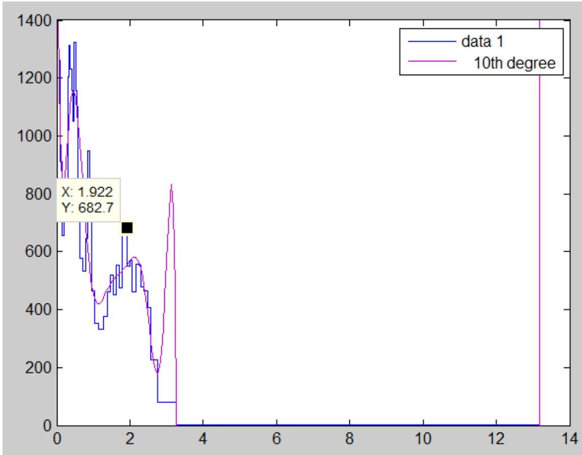
Figure 6: 120904162508 signal distribution after the DOF qualification step. A tenth degree poly fit is also shown that was used together with the data tip tool to identify a possible value for the peak (note that it is not the peak of the fit curve in this case).
