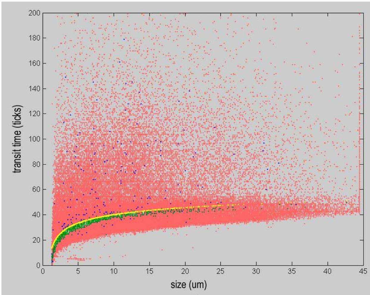
Figure 9: Half peak transit times versus size for the ICE-T FCDP research flight #4 on 7-12-2012 1441 to 1444 seconds of file (file RF4\_7-12-2011 110712175445\_frm\_1441\_to\_1444\_PBP). All
