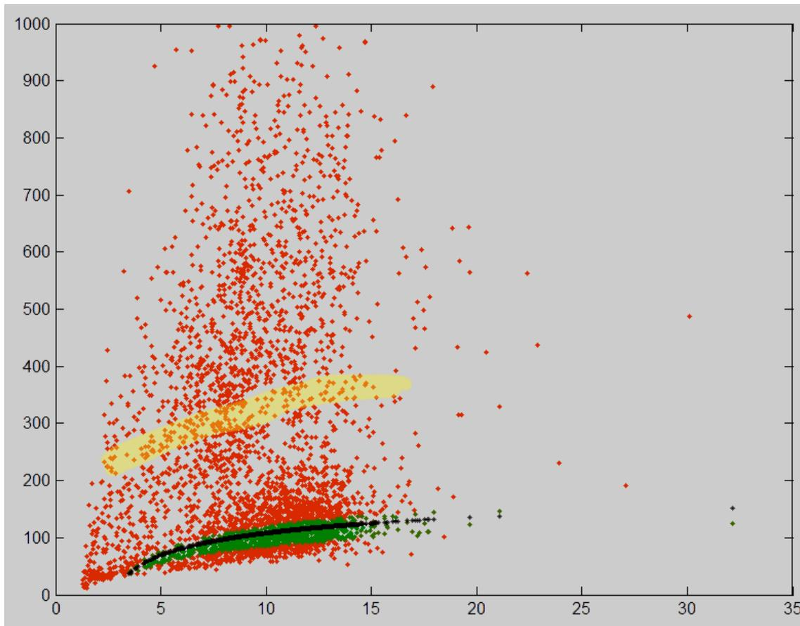
Figure 4: Half peak transit times versus size for 120904162226. Red are all data points just before the final transit time qualification processing steps. Green are the points remaining after the transit time qualification (TAS = 30 m/s). Black are the calculated transit time estimates. The yellow swath shows approximately the points that were transit time qualified (would have been green) when the TAS was set at 10 m/s.
