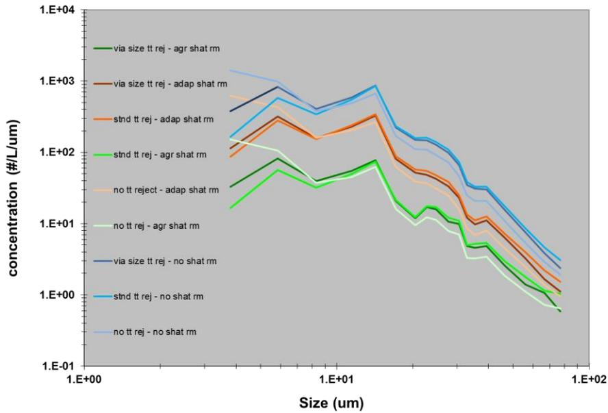
Figure 12: PSDs using various transit-time and shattering rejection options for the same data shown in Figs. 7 and 8.
