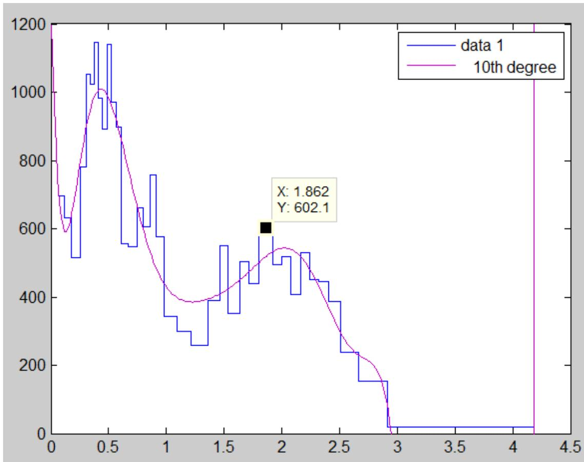
Figure 7: 120904162508 signal distribution after the half peak transit time versus full transit time qualification step (i.e. just before the final transit time qualification steps). A tenth degree poly fit is also shown that was used together with the data tip tool to identify a possible value for the peak (note that it is not the peak of the fit curve in this case).
