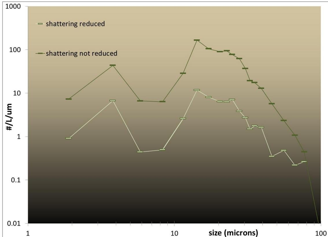
Figure 6: the final PSD produced with and without using the shattering reduction processing step. The data are from a period of large ice aggregates from 21:34:18–21:37:16UTC on 23 July 2010 (SPARTICUS).
