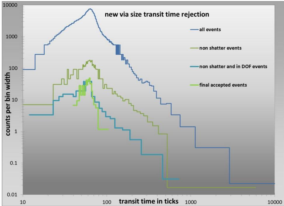
Figure 16: transit time distributions at various stages of the processing, indicating that the new via-size transit time rejection worked well here
