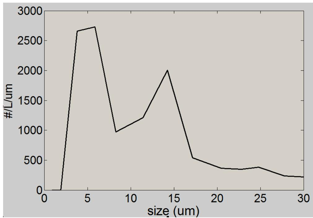
Figure A4: standard PSD, using the binning determined to account for the Mie bumps, for the data shown also in Figs. A2 and A3.
