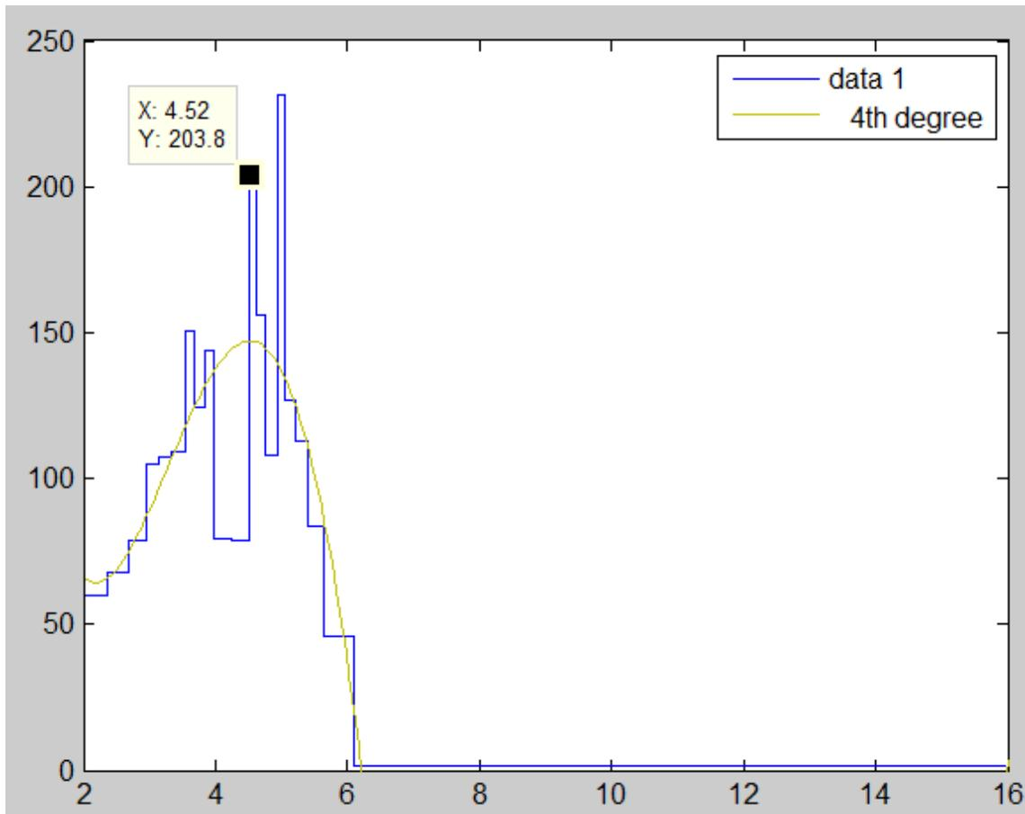
Figure 13: 120904162807 signal distribution after the DOF qualification step and after the small end was removed by using the noise filter. A fourth degree poly fit is also shown that was used together with the data tip tool to identify the value at the peak.
