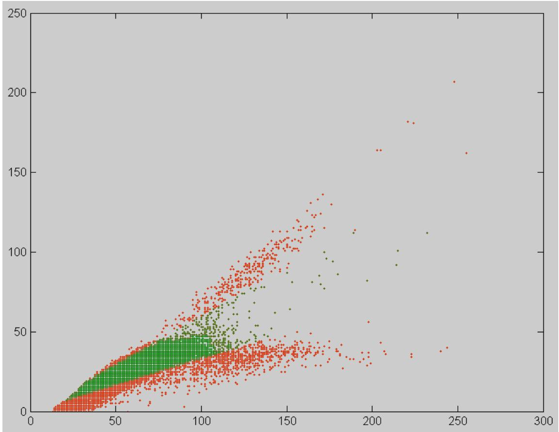
Figure 6: Half peak transit times versus full transit times for the period 14:45:23 - 14:45:30 (1603 - 1610 in seconds of file) FFSSP time. Red indicates before the half peak versus full transit time qualification while green above red indicates those points that remain after the half peak versus full transit time qualification.
