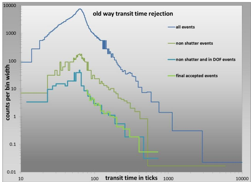
Figure 17: transit time distributions at various steps of the processing, indicating that the standard (mean transit time sets the cutoff) transit time rejection worked poorly here
