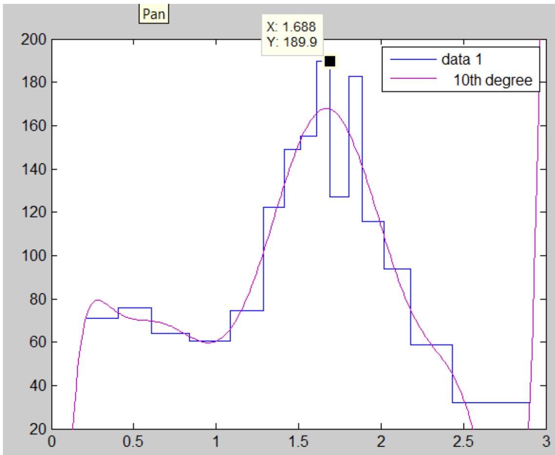
Figure 8: 120904162508 signal distribution after the final transit time qualification steps. A tenth degree poly fit is also shown that was used together with the data tip tool to identify the value at the peak.
