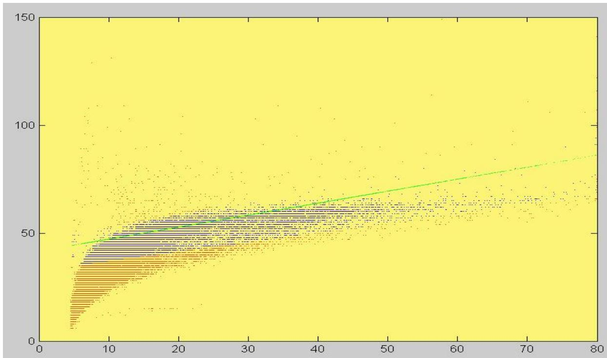
Figure 11: : Half peak transit times versus size for FFSP ICE-T data from 19 July 2011, 1431 to 1438 seconds of file, like figure 10 above but for a top hat beam profile model instead of the Gaussian beam model. It can be seen that there is room for improvement as the data is clearly nonlinear and the parameterization linear, though it works fairly well anyway in this case.
