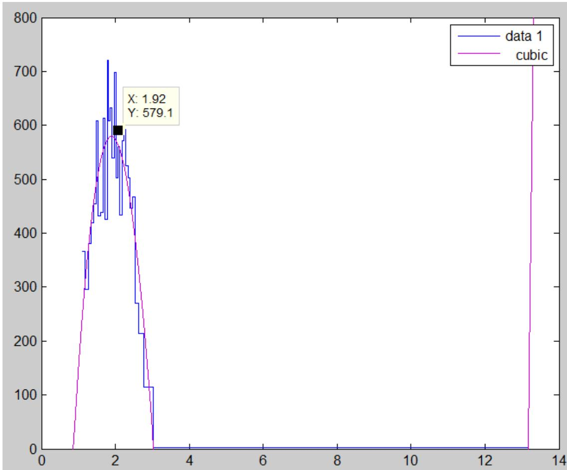
Figure 9: 120904162508 signal distribution after the DOF qualification step and after the small end was removed by using the noise filter. A cubic poly fit is also shown that was used together with the data tip tool to identify the value at the peak.
