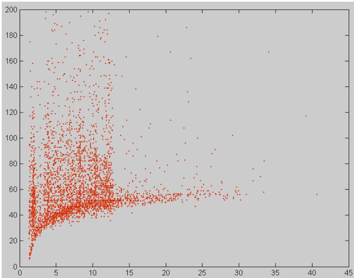
Figure 4: Half peak transit times versus size for the ICE-T FCDP 110712175445\_frm\_5228\_to\_5236\_PBP data after slit comparator qualification.
