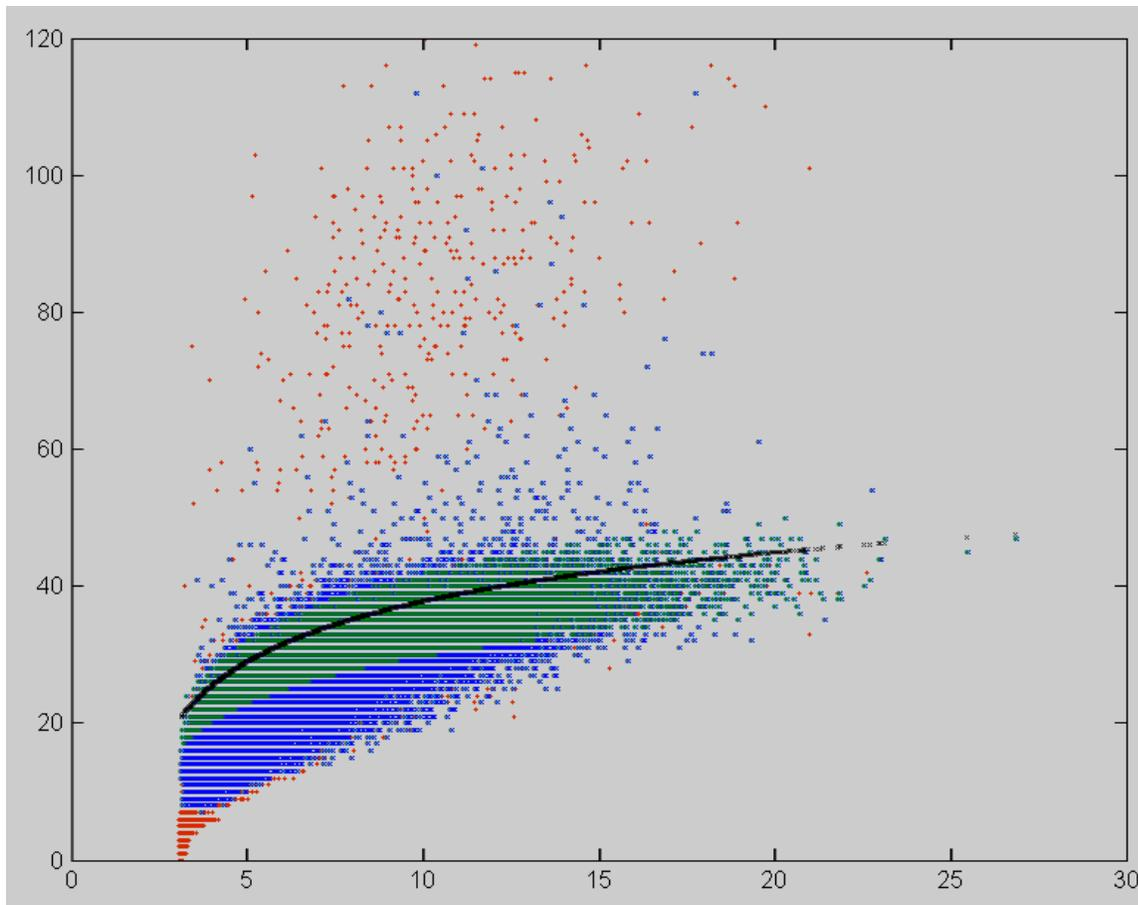
Figure 7: Transit time (y-axis in ticks) versus size (x-axis in um). Red indicates points after DOF qualification only, blue indicates after DOF and half peak versus full transit time qualification, green is after size dependent transit time qualification as well as the others.
