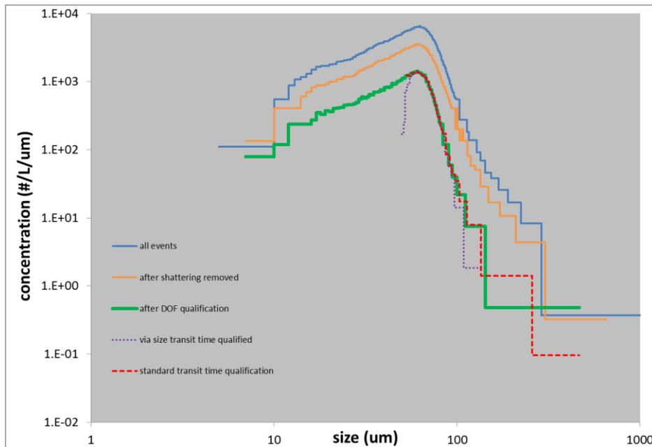
Figure 13: transit time distributions at various stages of the processing and for each of the final transit time qualification steps; via size and standard, for the same data as in Figs. 7, 8, and 12.
