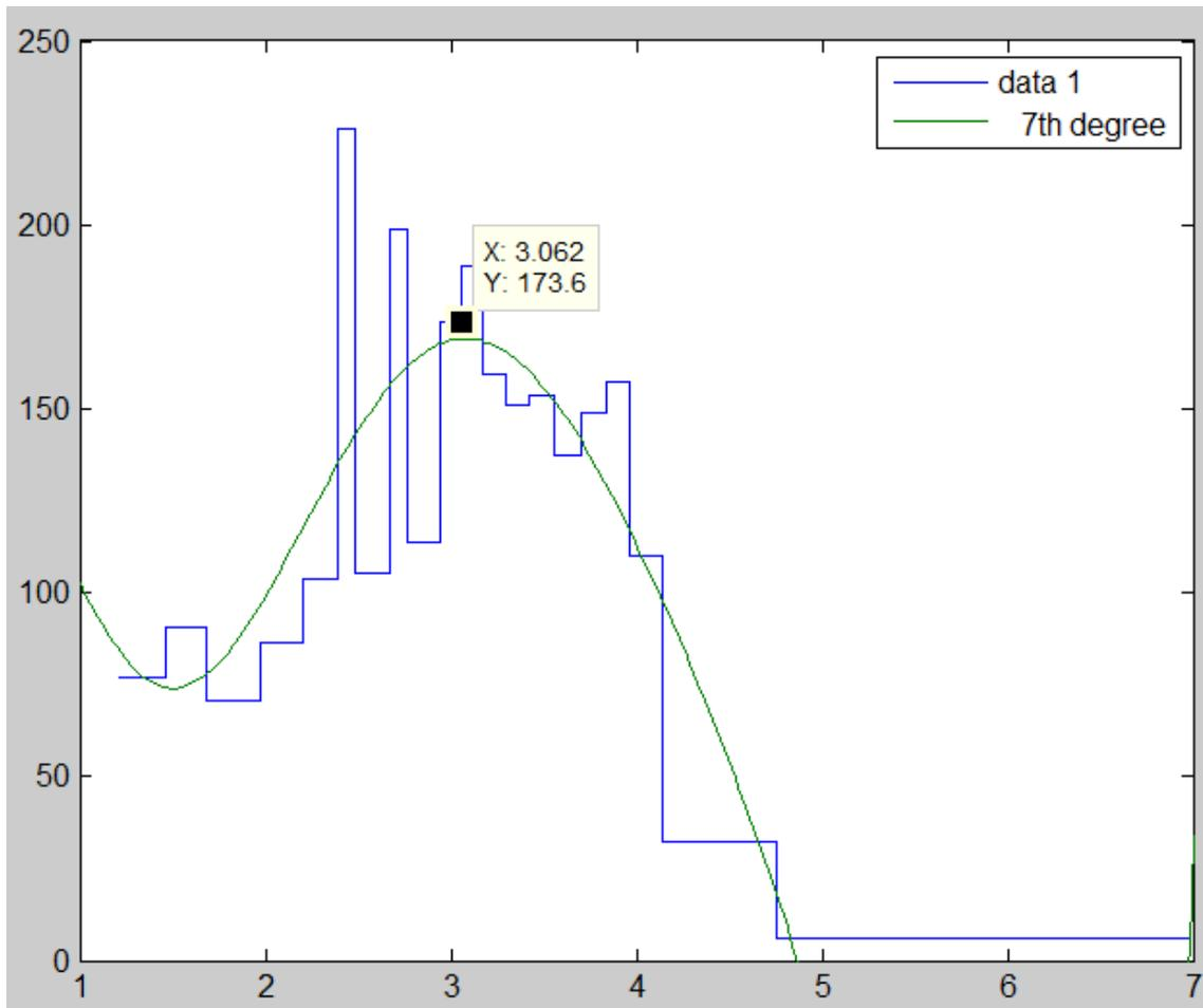
Figure 11: 120904162645 signal distribution after the DOF qualification step and after the small end was removed by using the noise filter. A seventh degree poly fit is also shown that was used together with the data tip tool to identify the value at the peak.
