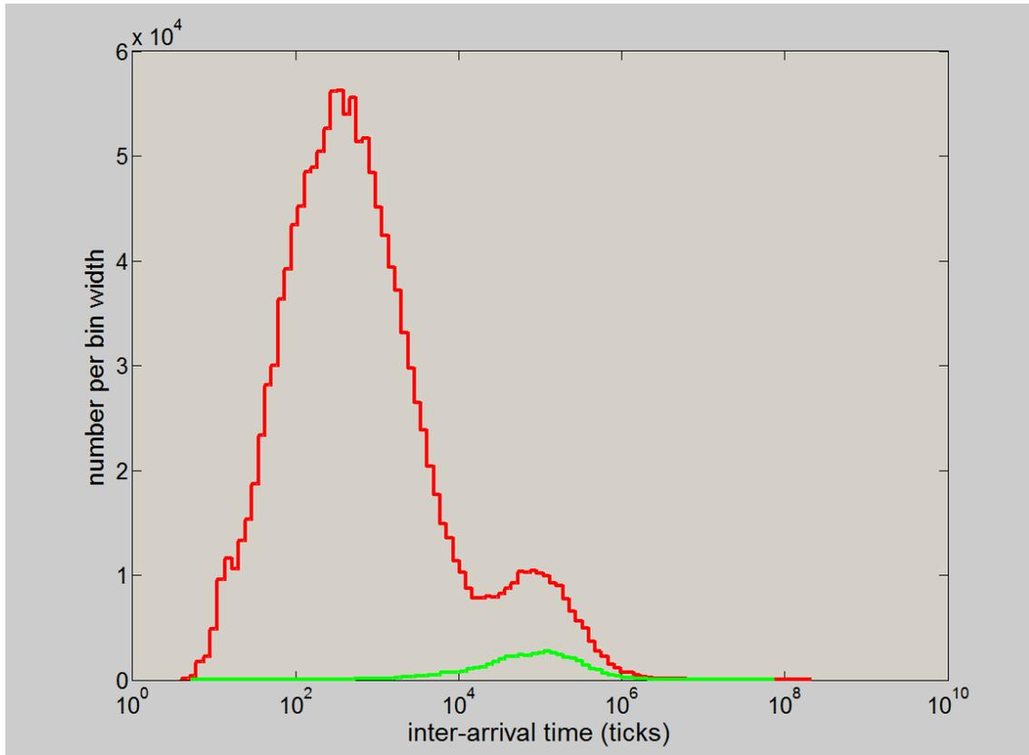
Figure 5: The inter-arrival time distributions before (red) and after (green) the shattering removal processing step. The data are from a period of large ice aggregates from 21:34:18–21:37:16UTC on 23 July 2010 (SPARTICUS).
