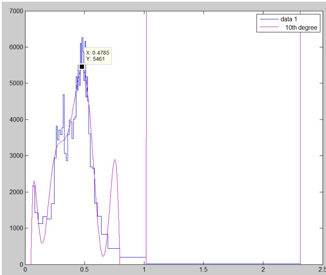
Figure 1b: 120904161915 signal distribution after the DOF qualification step. A tenth degree poly fit is also shown that was used together with the data tip tool to identify the value at the peak.
