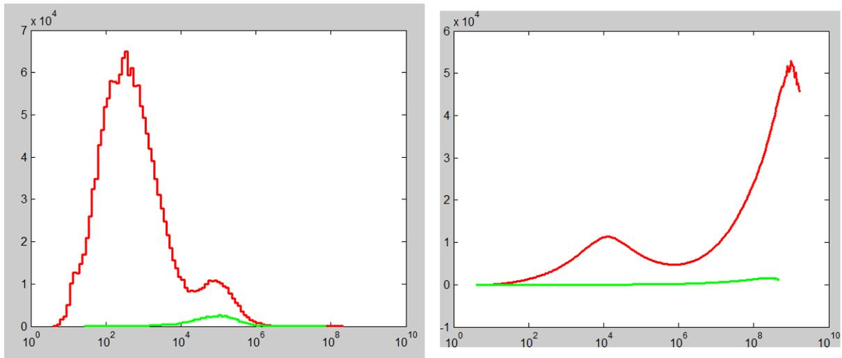
Figure 14: inter-arrival times (left) and fishing results (right) from just before (red) and after (green) the shattering removal (adaptive = aggressive in this case) step
