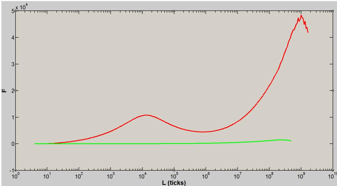
Figure 4: The results of the fishing test applied just before (red) and after (green) the shattering removal processing step. The data are from a period of large ice aggregates from 21:34:18–21:37:16UTC on 23 July 2010 (SPARTICUS).
