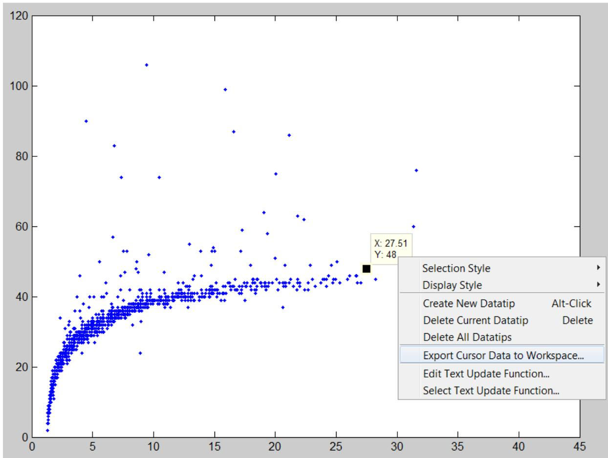
Figure 1: Half peak transit times versus size for the ICE-T FCDP RF4\_7-12-2011 110712175445\_frm\_1441\_to\_1444\_PBP, demonstrating the use of the data cursor to capture calibration data points.
